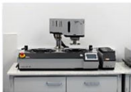
Sample preparation (grinding, polishing, electropolishing)
