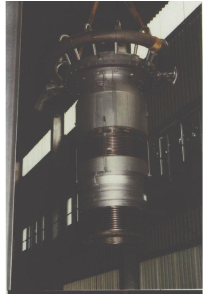
Core Connection System test tube flow diameter 700 mm
