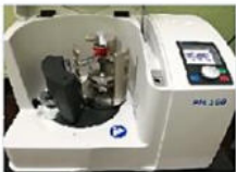
Milling in Planetary ball mill Rotation speed: 250 rpm Milling time: 10 / 20 / 30 / 40 h BPR: 5:1
