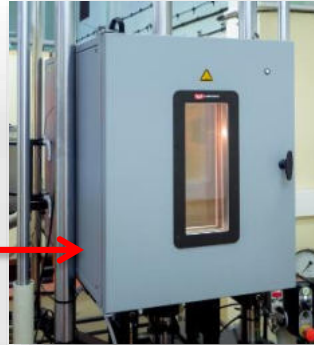
Temperature test chamber with cooling module Temperature range: from -150°C to +350°C
