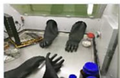
Powder mixing in Ar-atmosphere glovebox
