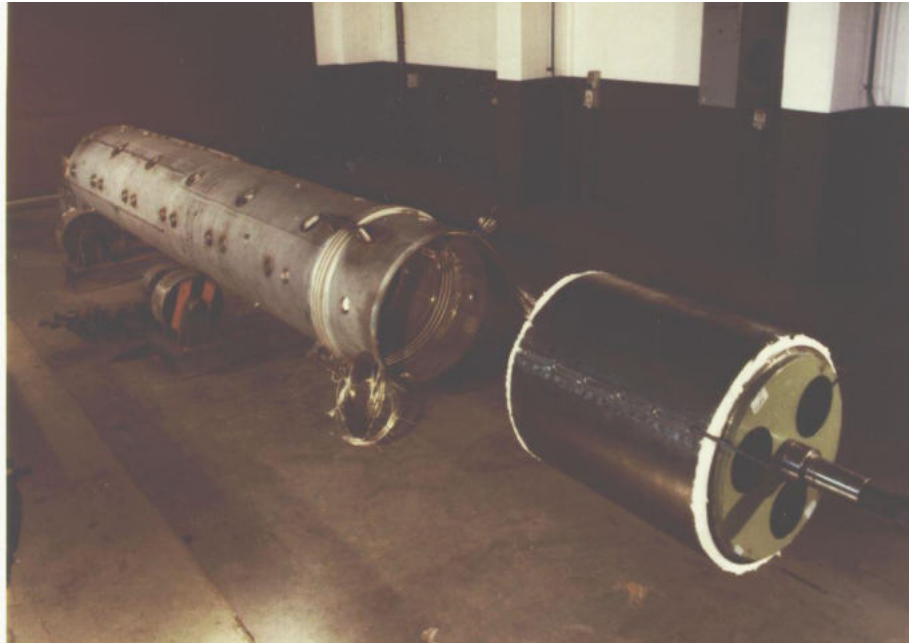
Horizontal test tube outer diameter 1020 mm wall thickness 20 mm flow diameter 700 mm
