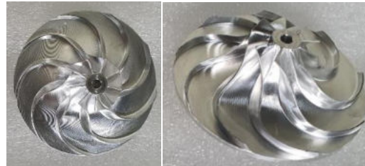
Compressor impeller with different backswep angle (50°, 70°)
