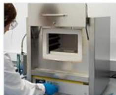
Annealing of samples Temperature: 1050 degree C Time: 12 h
