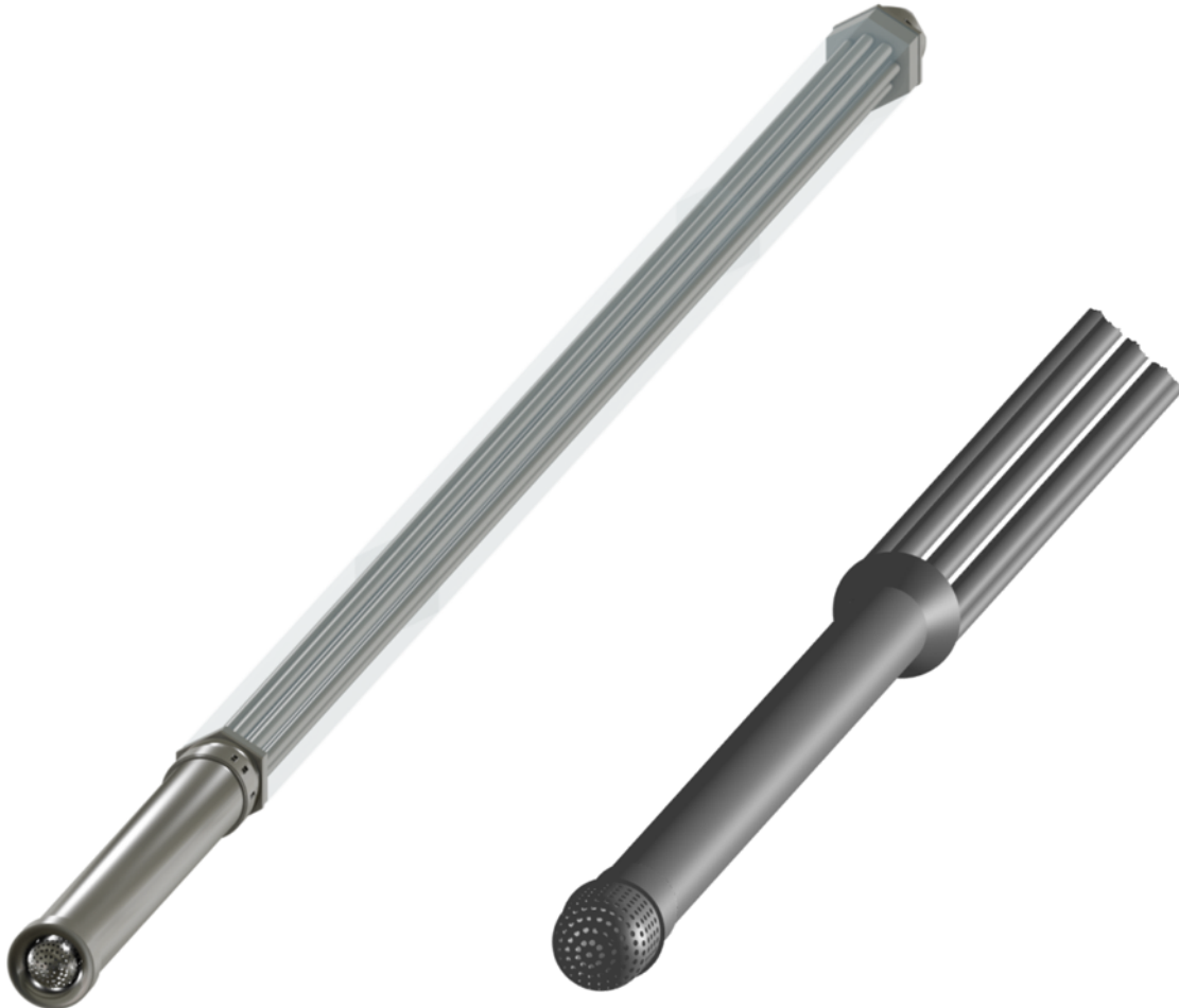
Figure 3: Design of reflector/shielding assembly [3]
