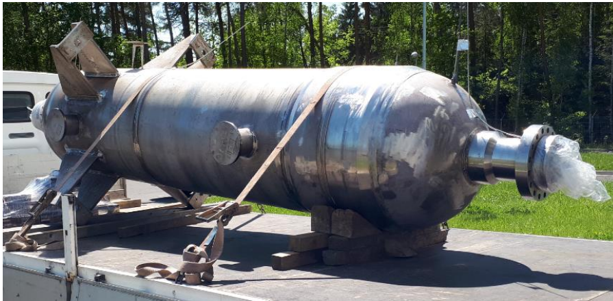
Figure 2-2: Primary heat exchanger of S-Allegro facility (transportation)
